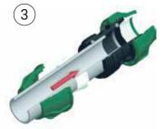
Insert the pipe into the fitting body and make sure the pipe crossed the O ring - gasket.
