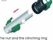
The nut and the clinching ring have to be pulled up on the pipe.
