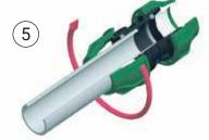
Pull back the nut and fully coil it up to the fitting.
