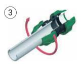
Fully coil back the nut to the fitting.
