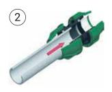
Insert the pipe into the fitting body and make sure the pipe crossed the O ring - gasket.
