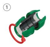
Limber up the nut, but do not remove it completely.
